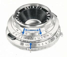
If the camera is focused on 10 feet the sharp zone will be from about 8 to 20 feet. In the above illustration arrows and dots have been included to make this point clearer and show how you can read off the depth of field from the focusing scale of your camera.
