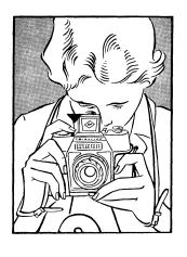
Another point in favour of the hood type of viewfinder is that you can aim the camera up in the air or downwards without twisting your body in any way. By using the sling you can also photograph satisfactorily in a crouching position. The Agfaflex can even be used for photographs in crowds by holding it over your head and viewing the subject on the ground-glass screen from below.
